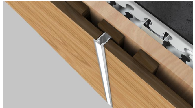
Example of application: wooden decorative board on the wall Cutout:W10*D12mm fixed by glass cement
